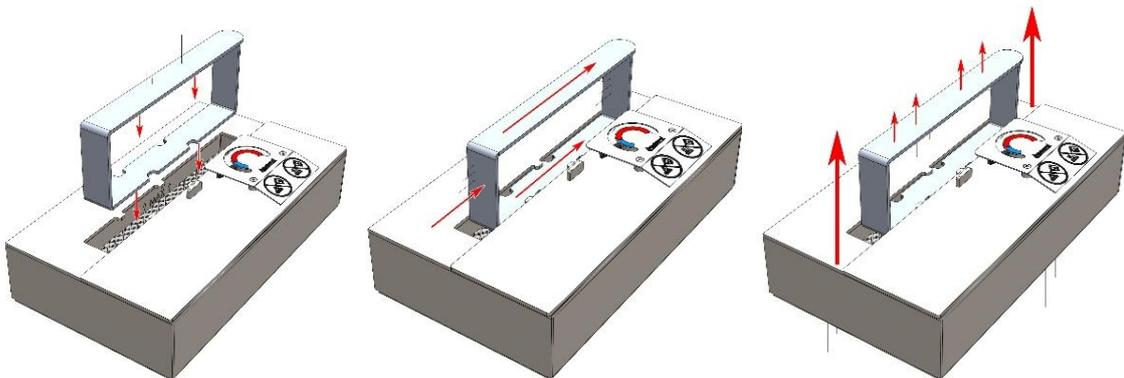
3. You can now remove the slider with the temperature indicator and grab the burner with your hands.
