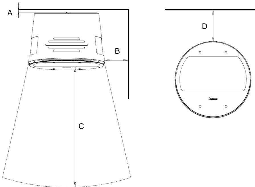
If the stove is being wall-mounted, it can only be mounted on a non-flammable wall. If the stove is placed on the metal foot, it should be placed on a non-flammable material. If the stove is positioned against a brick wall or other non-flammable material, there are no minimum distance requirements.
