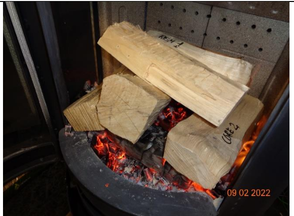
10) Placement of the LF fuel load in the firebox
