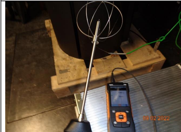
11) Intermediate air velocity measurement
