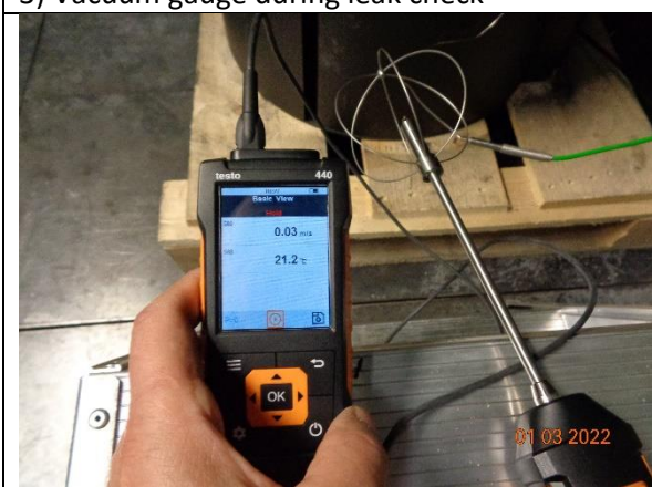
5) Air velocity measurement prior to the test
