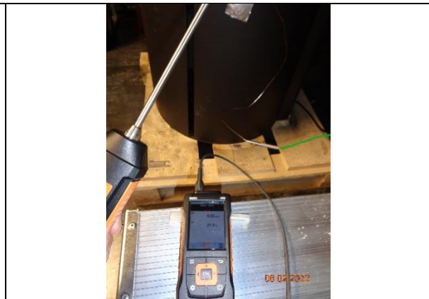
6) Air velocity measurement prior to ignition
