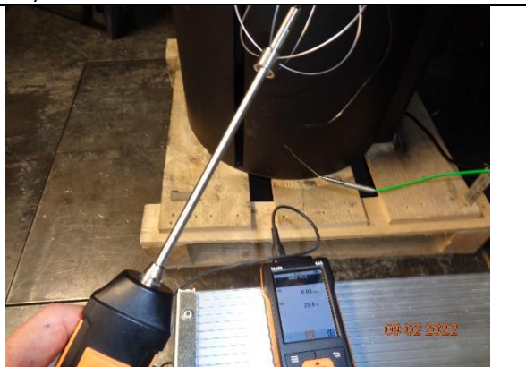
16) End of test air velocity measurement
