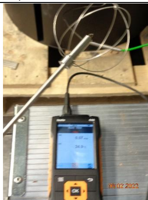
16) Post test air velocity measurement
