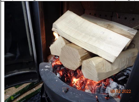
15) The LF fuel load in place in the firebox
