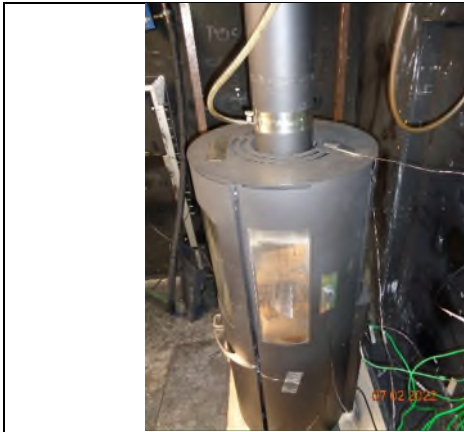
1) Installation of stove on the test rig inc TCs
