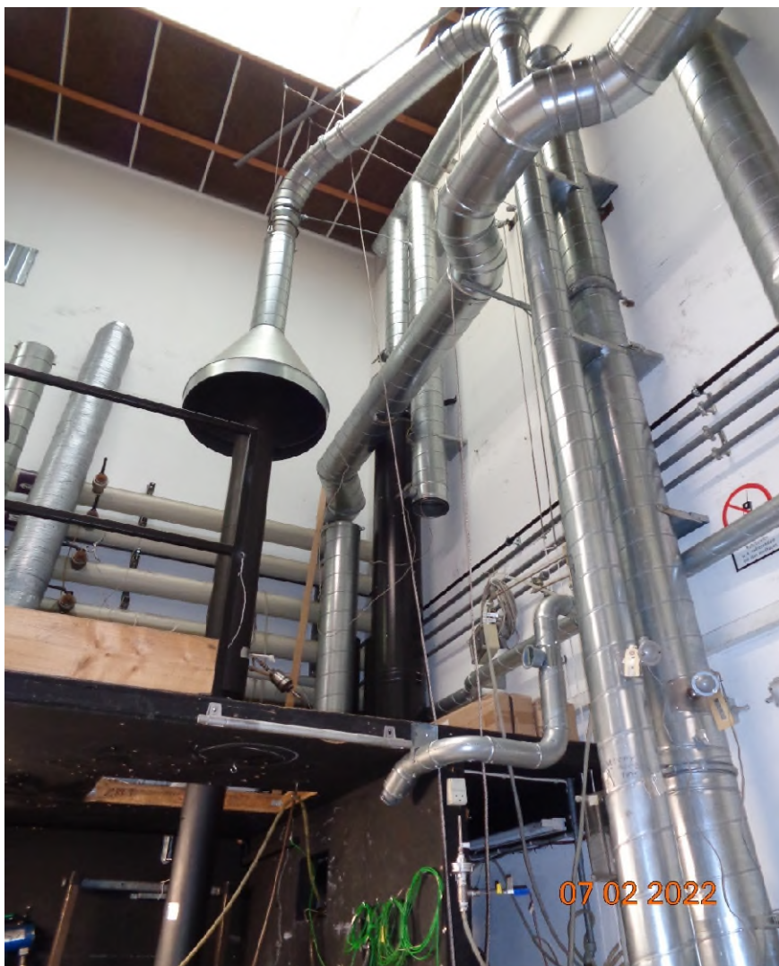
Details, Ø150 mm FFDT, extraction hood and insulated chimney part
