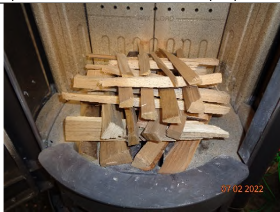
5) Placement of CS fuel load in the firebox
