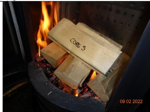
8) Placement of the HF fuel load in the firebox
