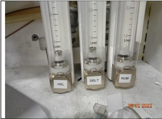
1) Morning sampling line leak check (zero flow)
