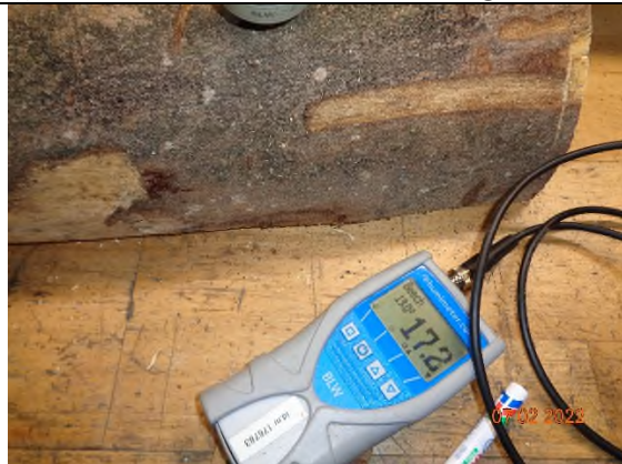
3) Measurement of fuel moisture (WB)
