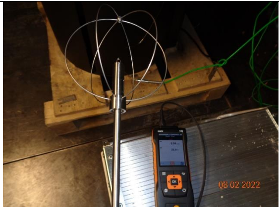
14) Intermediate air velocity measurement
