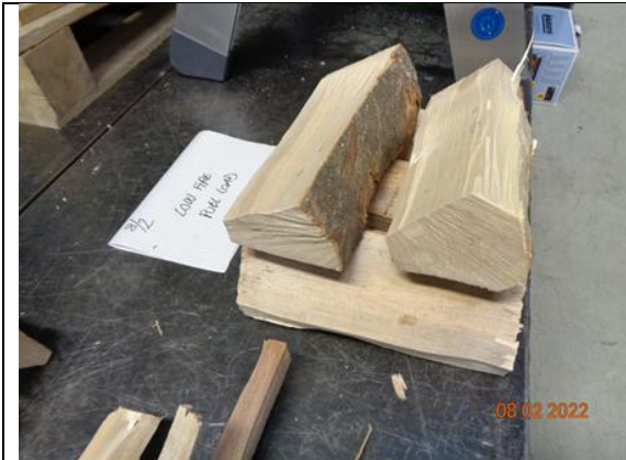
13) Arrangement of the LF fuel load (5 logs)
