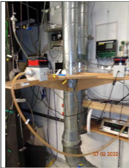
17) Temp controlled \varnothing 47 Pall filter holder arr.
