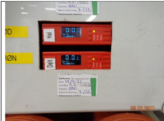
5) Morning sampling line leak check (zero flow)
