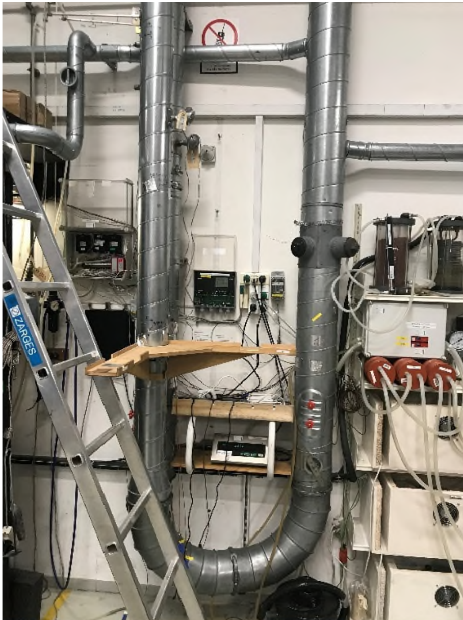
Details, pitot tube, temp sensor, sampling and traverse parts of the FFDT
