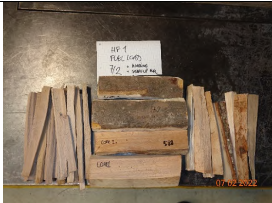
4) Arrangement of the entire HF + CS fuel load
