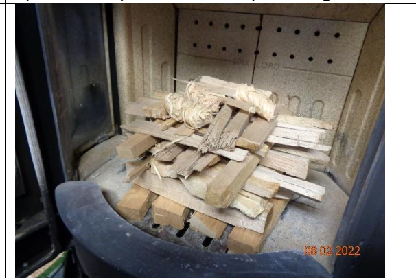
8) Arrangement of the CS fuel in the firebox
