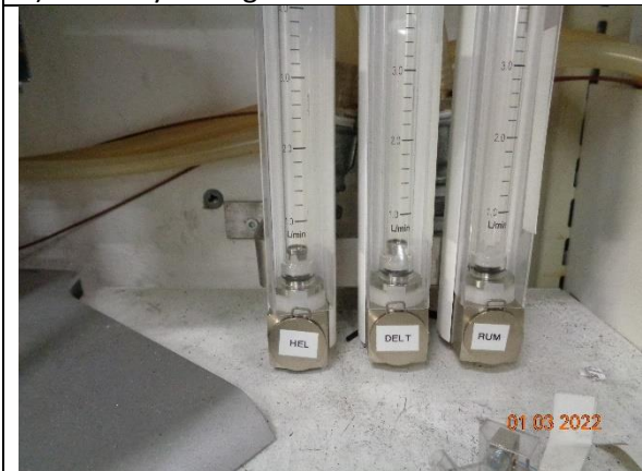
11) End of test leak check
