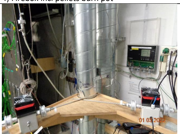
6) ASTM temp controlled sampling arr.
